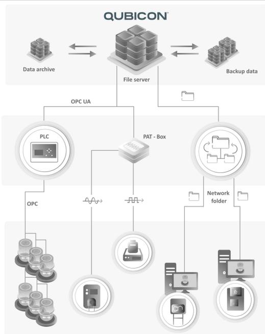
Figure 1: Schematic representation of the automation architecture at Ichnos. Devices can be connected to Qubicon either directly, through the PAT-Box or by utilizing the automated offline import.
